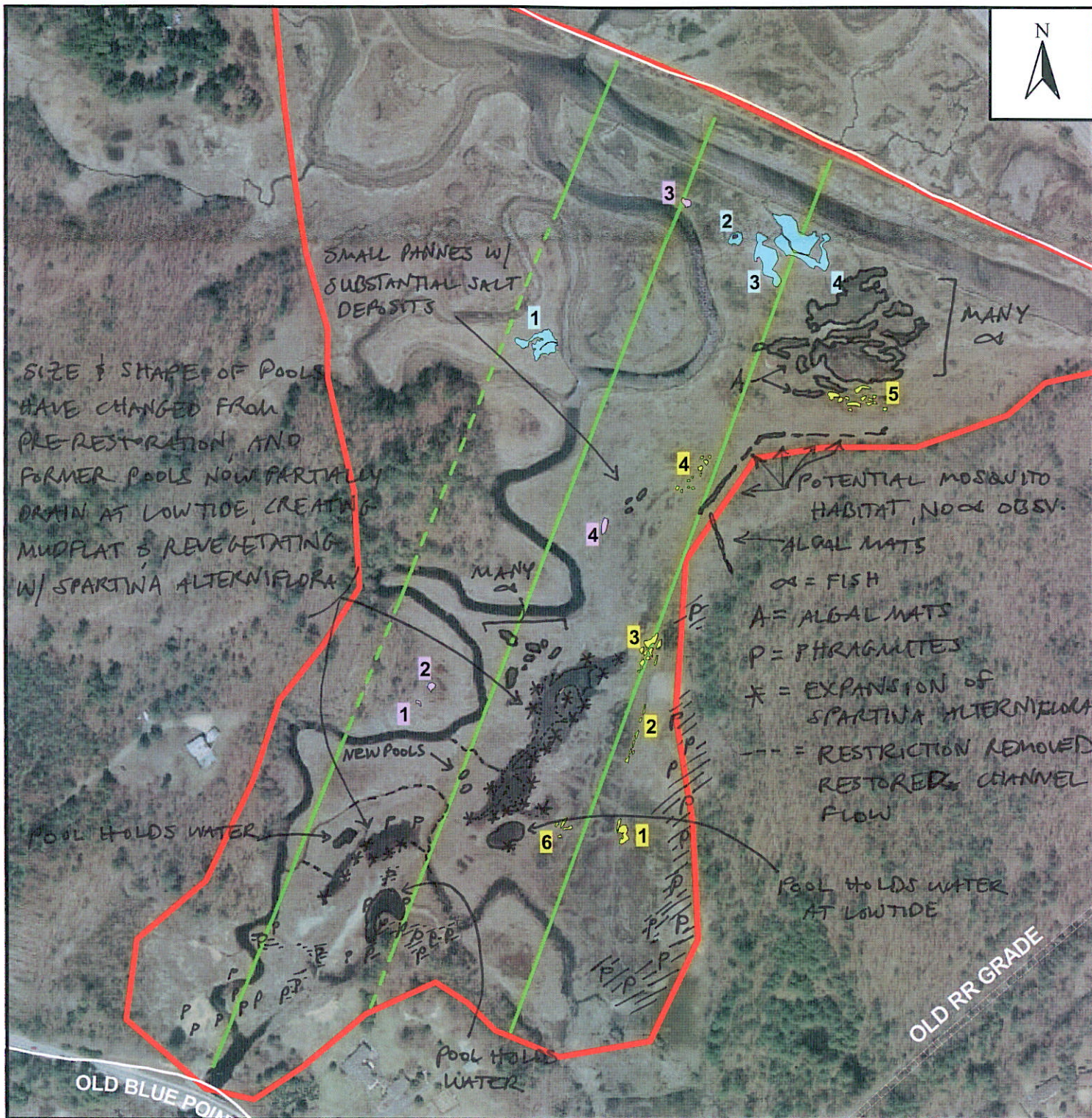
Figure 2. Site Assessment Transect Locations for Cascade Brook Salt Marsh Restoration Monitoring Project Scarborough, Maine.
